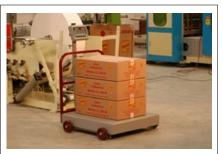
The EQM Series Receiving Scale features overload/impact protection and can be disassembled and used as a platform with remote indicator.
