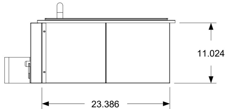
The dimensions shown are the actual physical dimensions of the Ice Chest. Additional clearances to the cabinetry are dependent on the tolerances of the cut-out. We recommend an additional .250 inches approximately per side but the openings can be made smaller if the tolerances are controlled.
