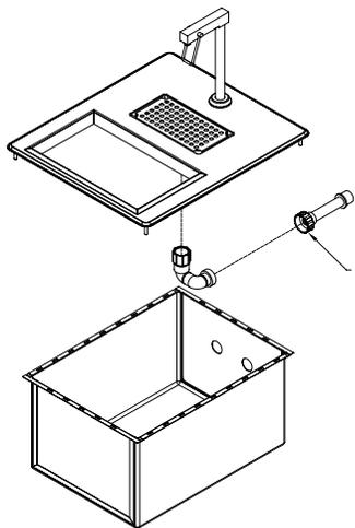
To install D-24-WSIBL2 unit into mounting surface, please loosen coupling and remove this section.
