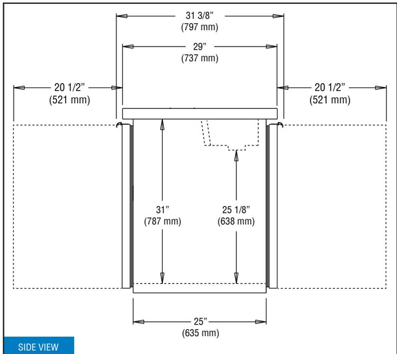
**IMPORTANT NOTE:** Models are completely front breathing and take in and exhaust air through the front grill. For proper operation, the area in front of the cabinet **must** not be obstructed in any way. A clearance of 3" on the sides is recommended.
