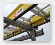
Ladder racks are a ladders worst enemy! Bauer has designed a protective rail guard that absorbs the abrasion and vibration that is harmful to ladders. Your ladders will last longer!
