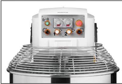
The stainless steel guard is ergonomically designed and completely safe. When guard is open at a 90° angle, the spiral dough mixer automatically stops working.
