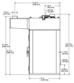
Height required to lift the oven from it's back, uncreated, without hood: 108" minimum.
