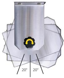
ADJUST AIR DISCHARGE BY +/- 20° ceiling mounting illustrated
