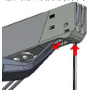
11. Pull the wire across the sealing bar straight and tight.
