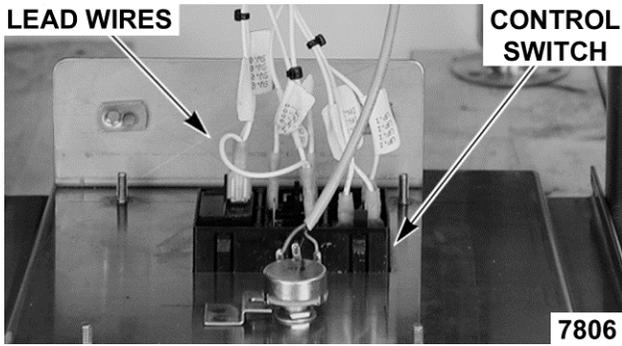
8. Pull temperature dial from potentiometer shaft and remove mounting nut.
