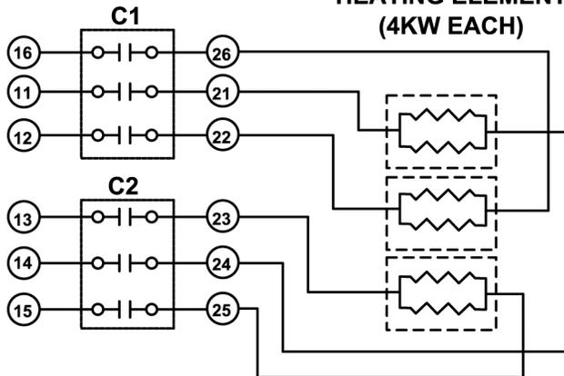
NOTE: See wiring diagram AI1378 for single and three phase power connections at terminal block.
