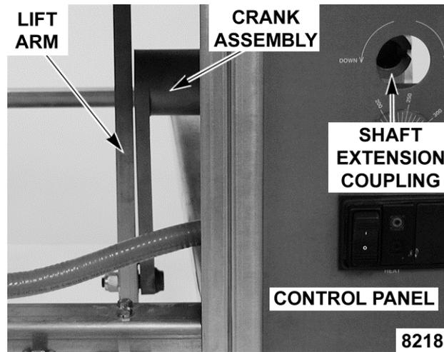
**NOTE:** On the bottom lift arm bushing, the bushing head must be positioned between the lift arm and the crank assembly to create approximately 1/32" spacing.
