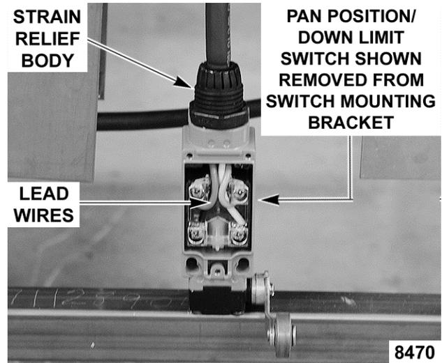
**NOTE:** When installing, ensure the o-ring seal is inserted into the strain relief body (around power cable) before tightening strain relief nut.
