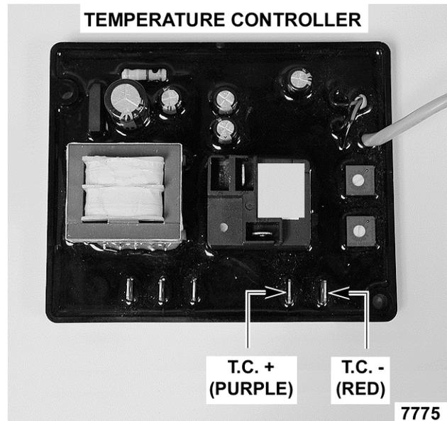
3. Check thermocouple for resistance.
