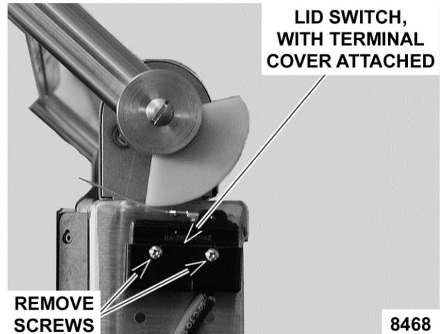
3. Lift terminal cover off switch body and disconnect lead wires.
