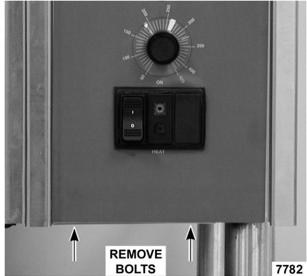
5. Tilt bottom of control panel outwards and pull down.
