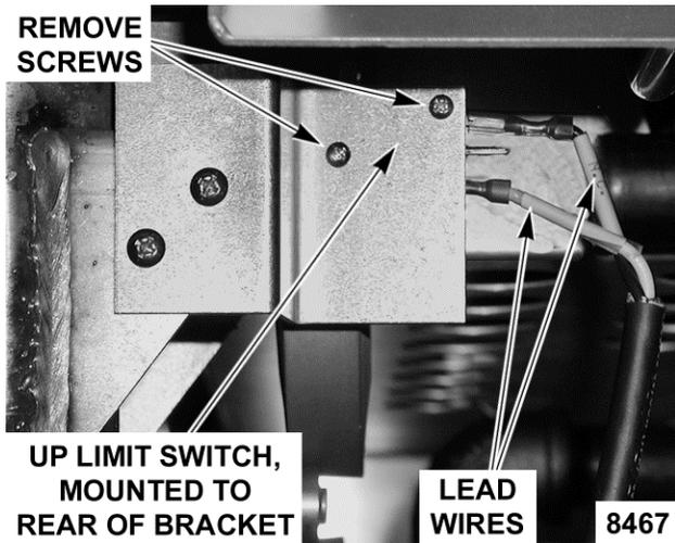
4. Reverse procedure to install and check for proper operation.
