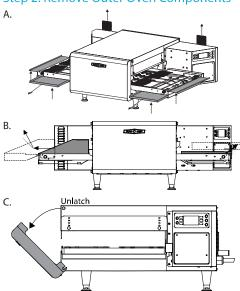
NOTE: Certain oven models are equipped with a side-swing front hatch. To remove the side-swing front hatch, unlatch and fully open it, then lift the front hatch upwards and off its hinges.
