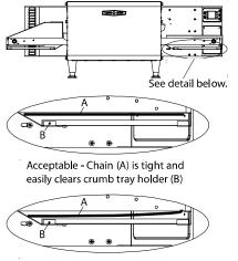
Call service to have link removed - Chain (A) is loose and risks contact with crumb tray holder (B)
