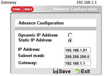
Press Save to save the changes and exit to return to the previous window. Your WLS scale is ready to communicate over a Wifi connection.
