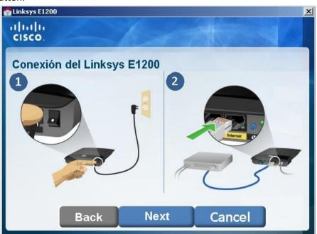
g) Make sure the connection is correct according to the image and press the Next button.
