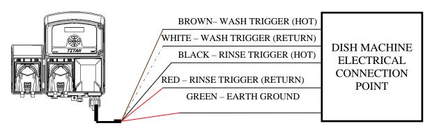
The following steps will help to insure the proper wiring of the unit. The unit should be triggered to power on from the dish machine that it is being used in conjunction with. DEMA Engineering does not recommend powering the unit separately from the dish machine. The following three steps will insure that the unit only receives power when it is necessary to have power to run the setup that is programmed in the unit.
