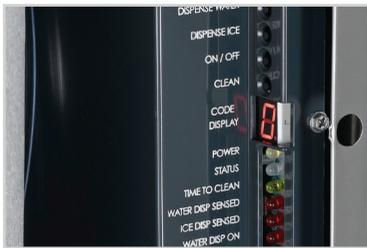
Internal LED indicator lights alert maintenance staff when it's time to descale, sanitize and more.
