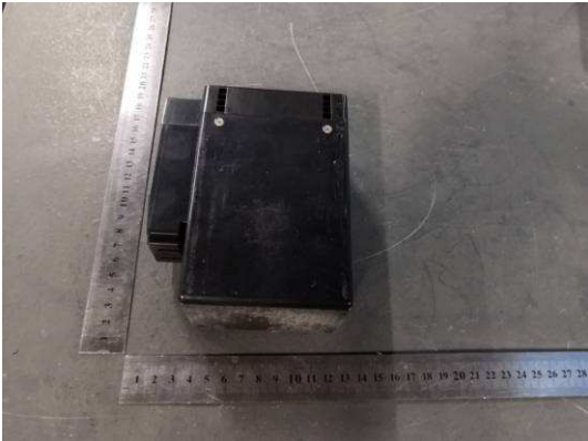
电池/ Battery(VACOBAT 22,2V 4,4Ah 97,68Wh)
