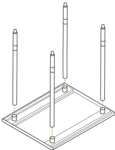
**3** Partially tighten the set screws—full tightening will come later.
