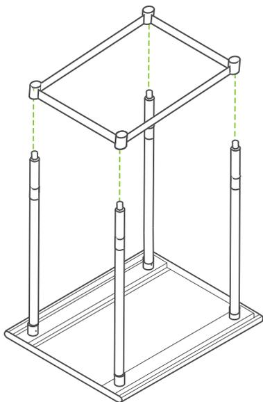
**6** Adjust the feet as needed to meet your height requirements or to compensate for uneven flooring.
