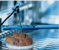
5. When loading the SelfCookingCenter<sup>®</sup> with **products of different sizes**, e.g., different pieces of meat, it is generally best to insert the probe into the smallest product. When using cooking processes followed by holding stage (Overnight Roasting, Braising, or Overnight Boiling), make sure that the holding stage is long enough that the larger products will reach the desired core temperature as well.
