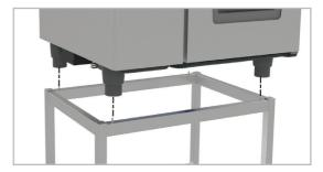
> Level the unit using the unit feet.
