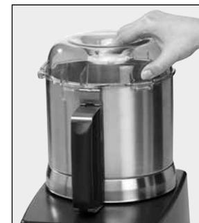
4) Note the plastic tab on the bowl lid. Place the lid on the bowl with the tab turned to the front and slightly to the left of the bowl handle; then, turn the lid back to the right until it comes to a stop with the tab over the bowl handle.
