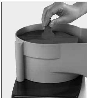
3) Place the white discharge plate onto the motor shaft. It should fall into place just off the bottom of the continuous feed attachment.
