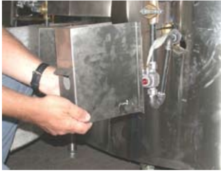
1. Remove the valve/control cover
