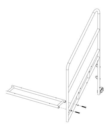
Once the two holes in the frame are aligned with two holes on the guardrail, place the provided washer on the M10 bolts and thread the bolts through the guardrail and thread it into the ends of the metal step frame.
