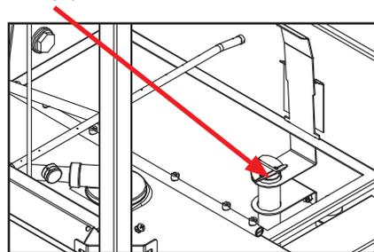
8. Once drained, put standpipe back in place and close door to refill the machine.
