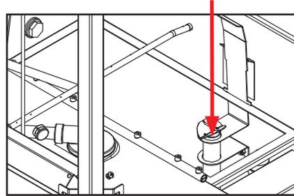
2. Allow machine to completely drain.
