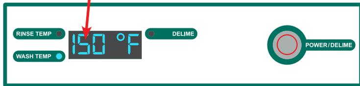
2. Once button is released, each press and release of button fewer than three seconds will advance wash temperature one degree at a time to a maximum of 170 °F, and will then roll over to 150 °F and advance up again.
