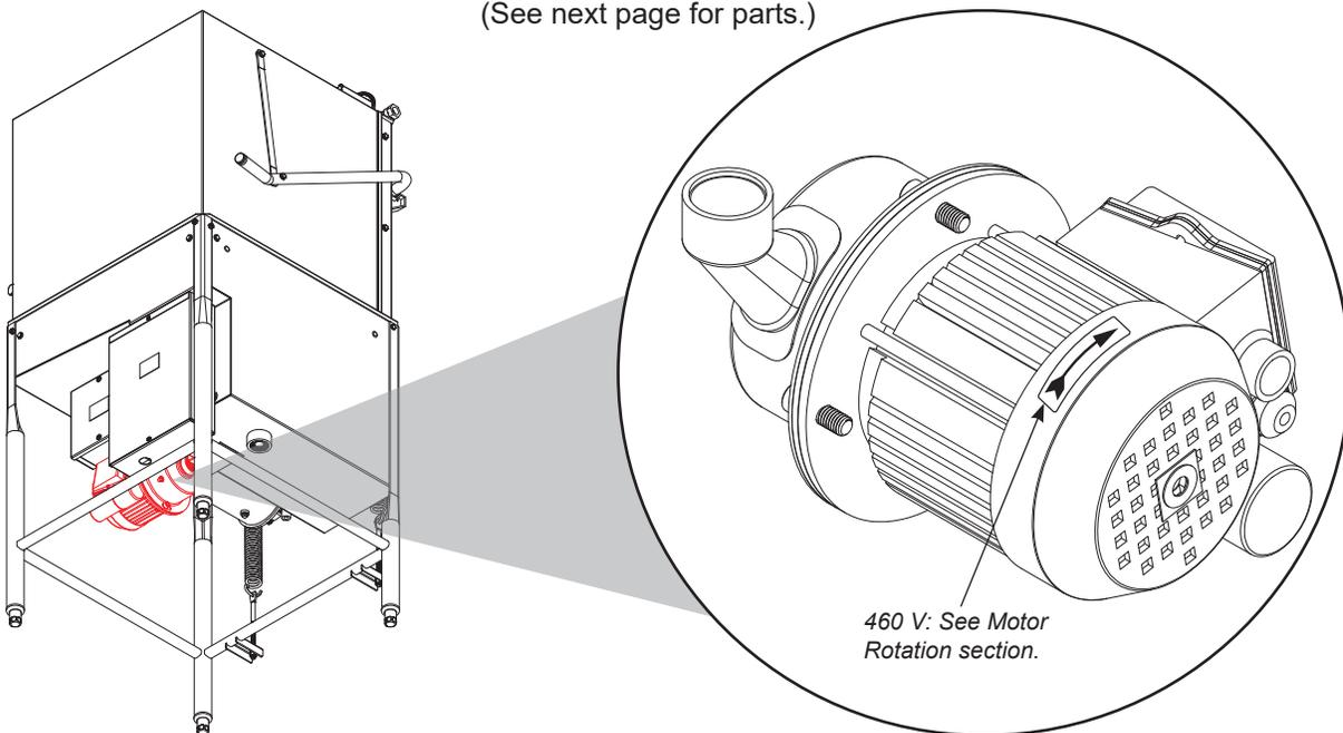
The models covered in this manual come supplied with various wash motor assemblies (a wash motor assembly includes the wash motor and the pump end), depending on the characteristics of the machine. To ensure you order the correct wash motor assembly for the model you are servicing, please refer to the following table:
