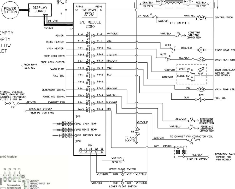
Connection Diagram for I/O Module
