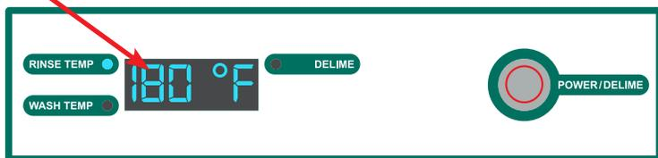
2. Each press and release of button fewer than three seconds will advance wash temperature one degree at a time to a maximum of 192 °F, and will then roll over to 180 °F and advance up again.
