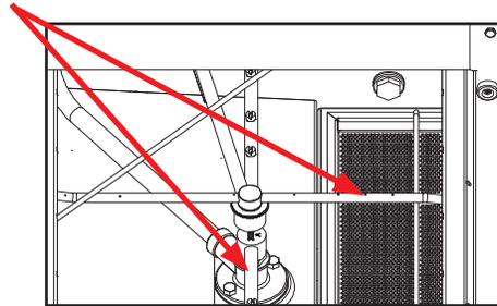
15. Ensure sump strainer and scrap screen are clean and securely in place.
