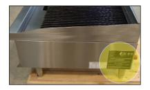
Item # 351CRCPG15 Model # CBR15 RADIANT CHARBROILER 15" Total BTU: 40,000 Gas Type: Natural gas Manifold Pressure: 6" WC Orffice Size: # 36 CLEARANCE REQUIREMENTS: Combustible Sides: 6" Combustible Back: 6" Serial # 110100001 Conforms to ANSI STD Z83.11-2016 and certified to CSA 1.8 STD-2016 Conforms to NSF / ANSI STD. 4
