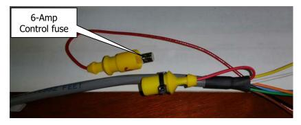
Gently pull the fuse holder apart as shown. Note that end with the black wire tie is designed to say in place tied to the cable.
