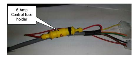
We suggest you unplug the 14-pin and 4-pin connectors from the controller to make it easier to access the fuse holder.
