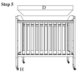
Place the mattress (D) onto the posture board (C)CAUTION: Use only mattress provided by manufacturer, which must be at least 38 inches long by 24 inches wide and not more than 3 inches thick.
