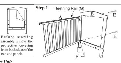
Note: That one side of each end panel has recessed drilled holes. These sides are facing outside of crib. Position side rail (A) with teething rail (G) up and warnings readable from out side of crib. Attach side rail (A) to end panel (B) using two hex bolts (E) and two barrel nuts (F). Tighten with allen wrench (I).
