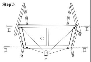
Lay crib down on the side rail and place posture board into position Insert four barrel nuts (F) into the barrel nut seats located under the posture board. Decide which height position you want the mattress support (C) to be (low, middle or high) See "WARNINGS". Attach mattress support (C) to the intended position to the end panels (B) using four hex bolts (E). Tighten with allen wrench (I).
