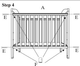
Position second side rail (A) with teething rail up and warnings readable from out side of crib. Attach side rail (A) to end panels (B) using four hex bolts (E) and four barrel nuts (F).
