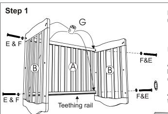
For step 1 it is easier to assemble the crib upside down on a padded surface.
