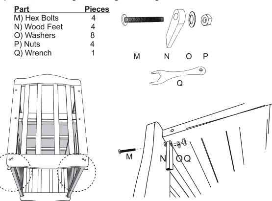
To disable the rocking feature of the crib. Attach the four wooden feet (N) to the inside of both of the headboards using the bolts, (M) washers (O) and nuts (Q).
