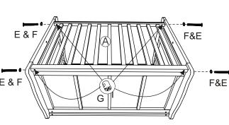
Insert 4 barrel nuts (I) into the remaining side rail ((A)
