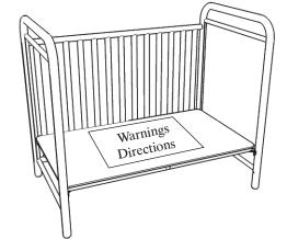
Align posture board (C) on top of posture board brackets (J) with 'WARNINGS/DIRECTIONS", label facing up.
