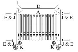
Attach remaining side rail (A) using bolts (E) and lock washers (J). Tighten all bolts at this time.
