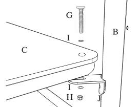
Attach each corner of posture board using Bolt (G), two washers (I) and lock nut(H) and tighten with phillips screw driver and wrench (M), as illustrated.
