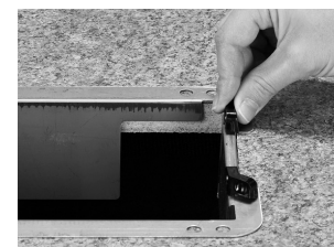
6. Alternate turning the black thumbscrews (D) clockwise until all four retainer paddles (C) are firmly engaged against the underside of the counter. Caution – Do not over tighten the thumbscrews as this may cause permanent damage to the mounting adapter.
