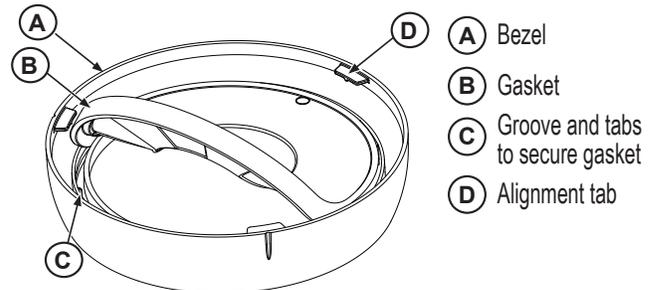
5. Install the bezel with gasket onto the tube.
