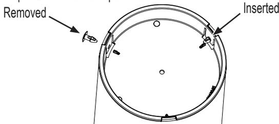
2. Remove the bottom plug, spring, and push plate from the tube.
