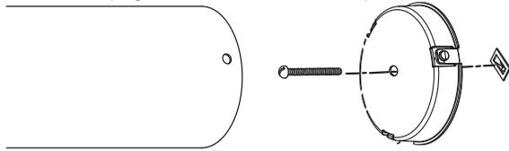
**NOTICE:** The screw must extend approximately 9/16" (14.2 mm) past the cabinet. Depending on installation, a longer screw may be required.
