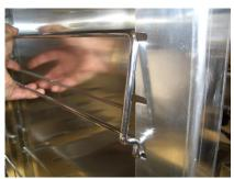
TILT THE RUNNER UP AND ENGAGE BOTH ENDS TOGETHER. DO NOT HAVE ONE SIDE ENGAGED LESS THAN THE OTHER.
