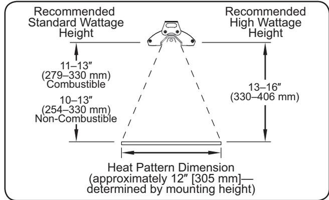
Recommended Element Height for the GR5A Series in all widths
