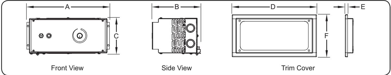
*NOTE: Make sure the control box installation location provides enough space behind the vertical surface for the depth of the control box and electrical connections.*
