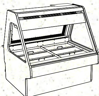
Model GMG4 Seafood Case: Remote Unit Rear Sliding Doors Removed. Ice Pans Used (Instead of Wire Racks as used in Meat Case Models GMG6, GMG8 and GMG12)
