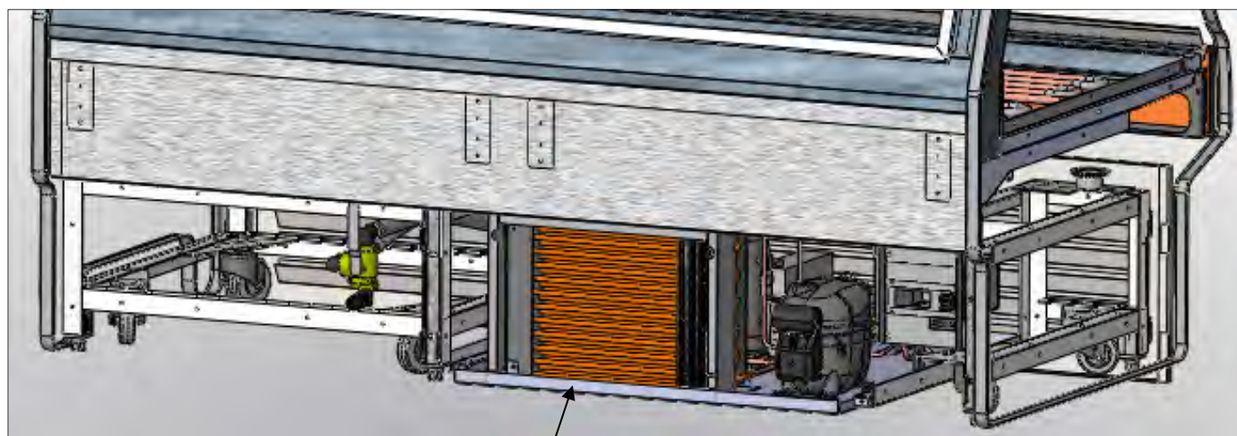
Refrigeration Package (Rear Grille Removed For Illustrative Purposes Only)
