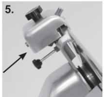
5. Remove the knife sharpener. Loosen the screw on the neck of sharpener then lift the knife sharpener off and away from the slicer.
