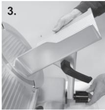
3. Remove the food chute from the slicer by loosening the food chute knob on the chute arm. **Note:** The chute release knob is not designed to come completely off. Lift the food chute off the chute arm.
