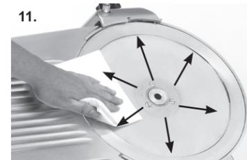
11. Carefully wash the top and bottom of the knife by wiping from the center of the knife outward.
