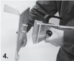
4. Disassemble the food chute. Using the knob on the back of the chute, unscrew the food chute into three separate pieces.
