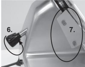
7. Remove the slice deflector by loosening the screw knobs.
