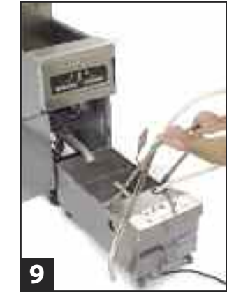
9 Position filter securely under the drain pipe.
