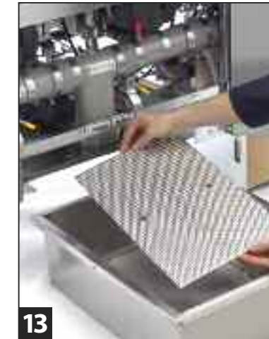
13 Return the filter screen to the filter pan and be sure that it is securely in place.
