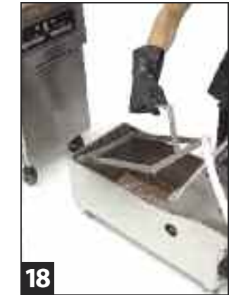
18 Remove and wipe off hold-down ring with paper towels.
