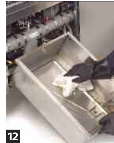
12 Wipe out filter pan with paper towels.
