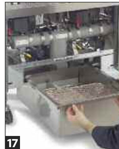
17 Slide filter pan back in place.
