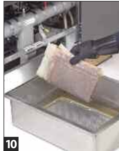
10 Remove and discard used filter paper.
