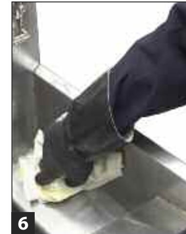
6 Turn off filter pump (yellow handle). Wipe out frypot with paper towels.
