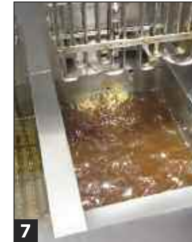
7 Close drain valve (red handle). Turn ON filter pump (yellow handle) and return filtered oil to the frypot. Allow oil to bubble for 15-30 seconds to clear return lines of oil.
