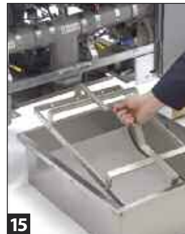
15 Make a good seal by placing hold-down ring over filter paper securing paper evenly and completely around all sides of the filter screen.
