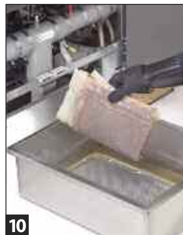
10 Remove and discard used filter paper.
