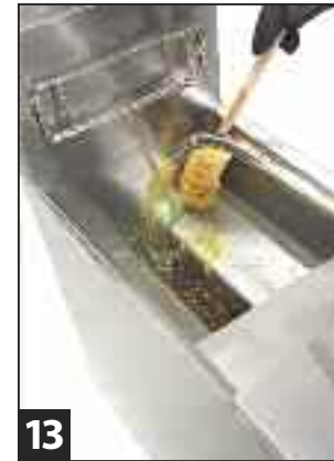
13 Use filter wand and fryer brush to remove crumbs from frypot sides and bottom.
