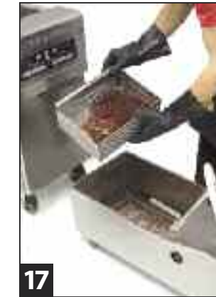
17 Remove, empty and wipe off crumb tray with paper towels. Discard crumbs into a fireproof container.
