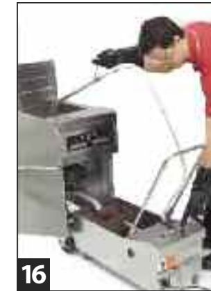
16 When all the oil is returned to the frypot, turn off the filter pump and unplug the filter power cord.
