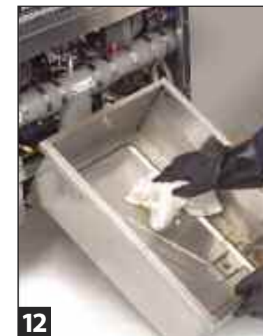
12 Wipe out filter pan with paper towels.
