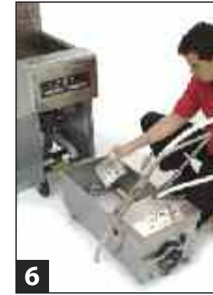
6 Replace hold down ring. Sprinkle one filter powder packet (1 cup) over filter paper.
