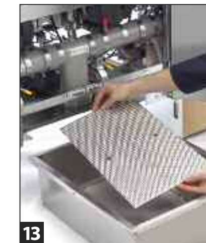
13 Return the filter screen to the filter pan and be sure that it is securely in place.
