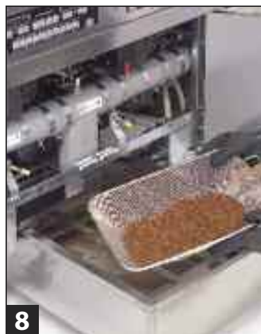
8 Turn off filter pump (yellow handle) and pull out filter pan. Remove, empty and wipe off crumb tray with paper towels. Discard crumbs into a fireproof container.
