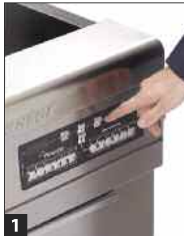
1 For all built-in fryers except fryers with the 3000 Controller, press OFF button to stop cooking cycle. Filtration works best when done near cooking setpoint temperature.
