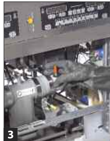
3 Make sure the filter pan is clean and prepared for filtering. Open the drain valve (red handle) and allow oil to drain into filter pan.
