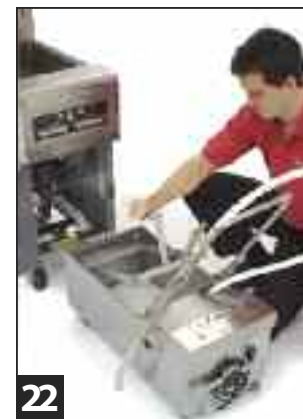
22 After filter parts have cooled to the touch, return the filter screen (making sure it is securely in place), hold-down ring, crumb tray, and lid to the filter pan.
