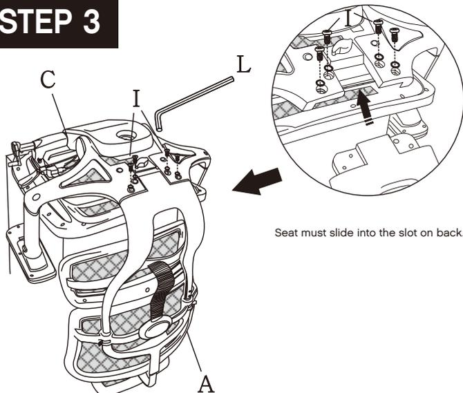
Seat must slide into the slot on back.
