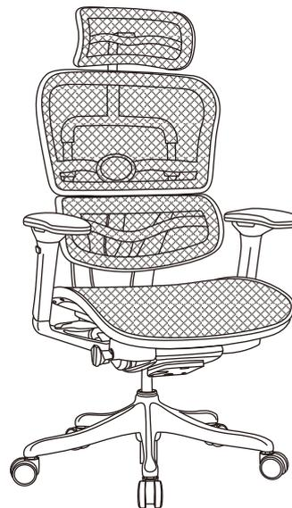
Now turn the assembled seat upright and locate the center hole of the Mechanism over the Seat Post. Push down firmly until the connection is secure.
