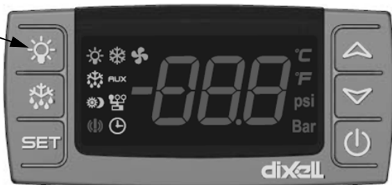
Light Bulb Icon Sample Dixell® XM670K/XM679K Controller Shown
