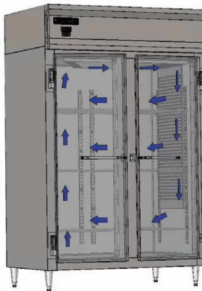
Top and Side Air Distribution Ducts
