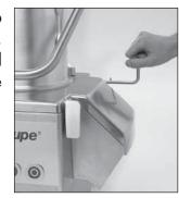
**2** Slide the hinge pin into the slots provided at the back of the motor base. Next, lock the lid onto the motor unit using the locking handle.
