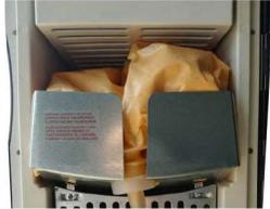
5. Guide the tube through the pump slot from top to bottom.
