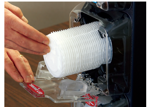
Illustration C Lids are uniform and evenly spaced right out of the sleeve. They will dispense very well.
