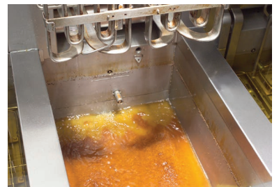
Built-in filtration rear flush moves crumbs to drain valve
