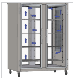
Plug refrigeration air flow
