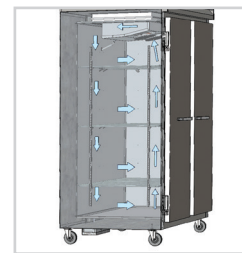
Modular refrigeration air flow
