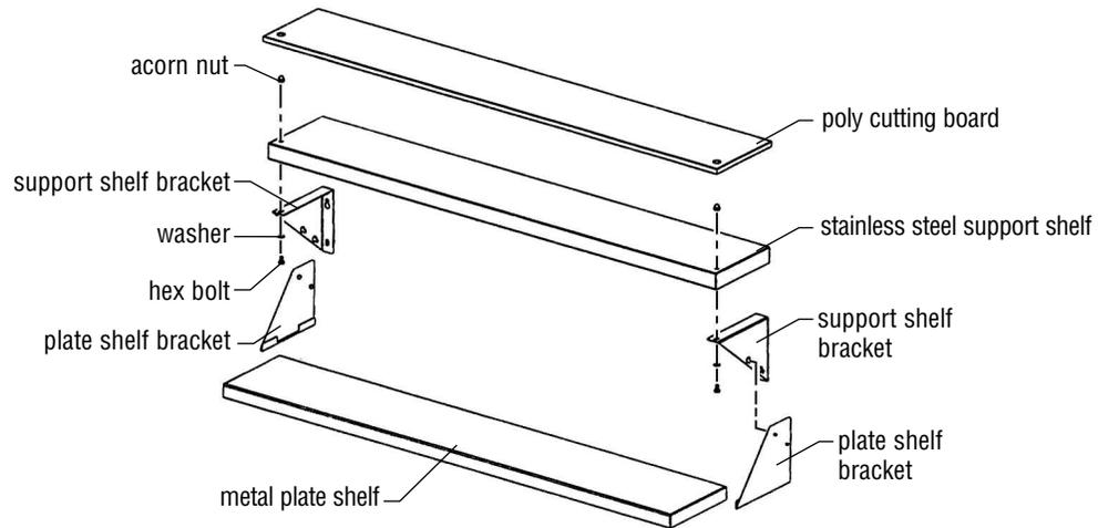
1. Attach shelf support brackets to support shelf, using acorn nuts, washers, bolts and predrilled holes. Note: acorn nuts must be at the top.
