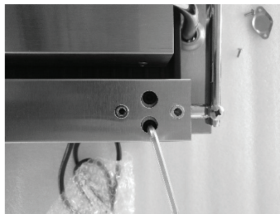
Step 2 - Using an Allen wrench, adjust the tightness to feel. Open and shut the top shell until the tightness feels natural while opening closing the lid. Your manual bag includes this tool and grease. Add the grease while moving the top shell to lubricate the hinge.
