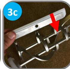
d. Insert beater assemblies into cylinders, *making sure beater shoes stay in place*; turn assemblies until they engage the drive shaft keys and no longer turn 360°
