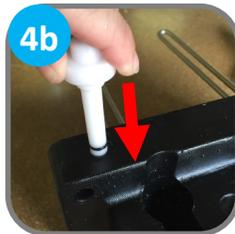
c. Insert draw valves into dispensing door, O-rings-first; *middle draw valve goes in the middle and slots face outward*
