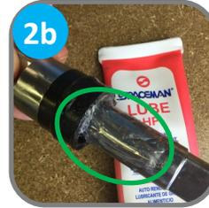
c. Insert drive shafts into rear shell bearings at the back of the cylinders, and turn them until the key engages firmly into the socket (when inserted correctly, the drive shaft will no longer turn 360°)
