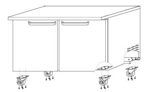
Note: The casters with brakes should be installed to the front of the cabinet.
