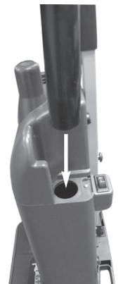
**6** Attach cord holder to short machine cord and 50 foot cord
