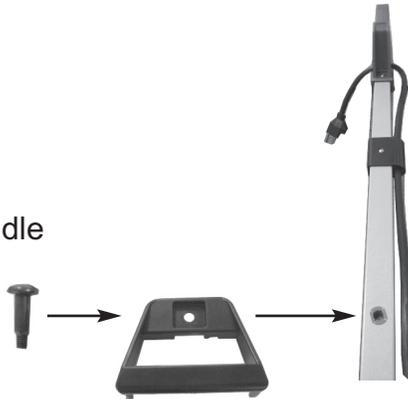
**3** Align with hole in center of vacuum handle and push through into vacuum bag housing. Tighten bolt with screwdriver until it is completely secured.
