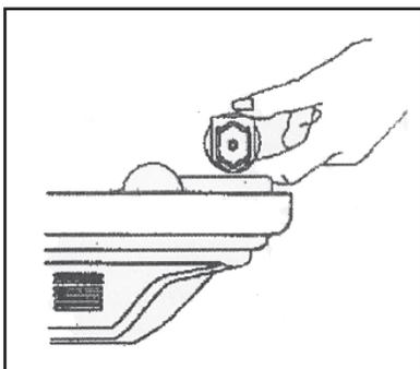
**E.** Pull belt over pulley and set. Rotate pulley to make sure belt is riding smooth on motor pulley.
