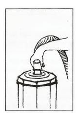
Put backpack on and adjust shoulder straps and waist belt until backpack is comfortable. Harness is made for any custom fit. Attached hose to commercial wand. Attach desired tool to bottom of wand by loosening nut and pushing in tool. Tighten nut until tool is in place. Tool will swivel when using side to side motion. Never take nut off wand or risk losing metal ring inside the nut. The function of the metal ring is to hold tool in place in its slotted groove.
