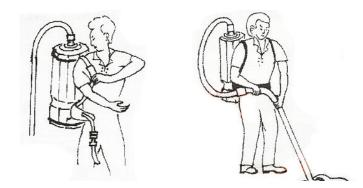
Your LAVEX JANITORIAL backpack comes with a switch box that has the on/off switch, a power nozzle receptacle and power receptacle all in one. It has velcro and a strap on the side so it can be removed from the waist belt and put back at a comfortable setting for the user. Simply push rocker switch to on or off position to operate.
